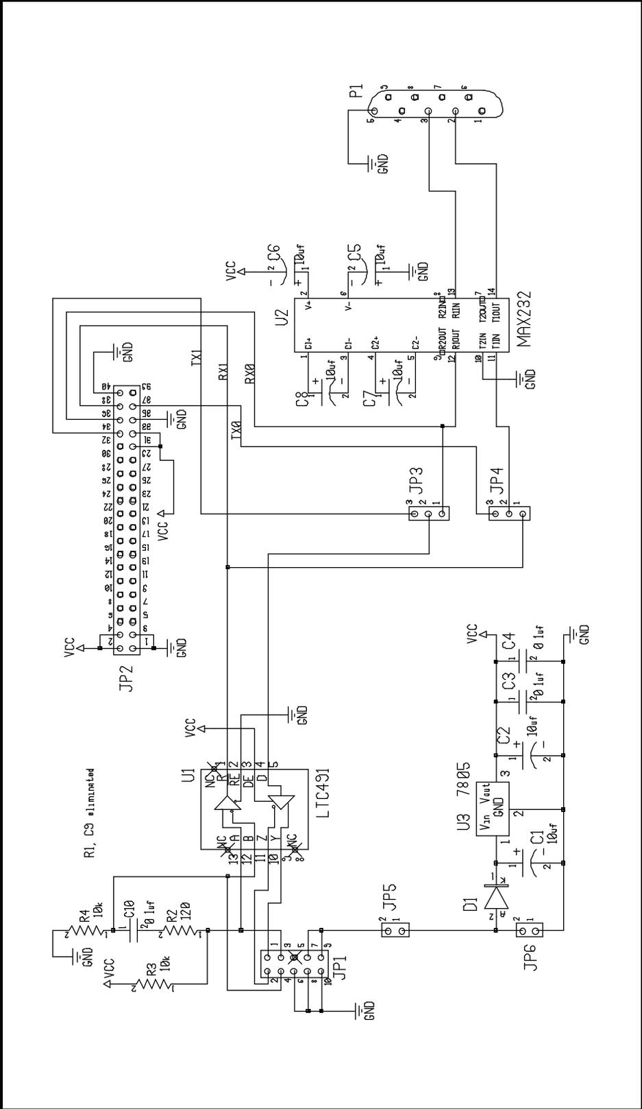
Figure 3 - Z232-485 Converter Board Schematic
