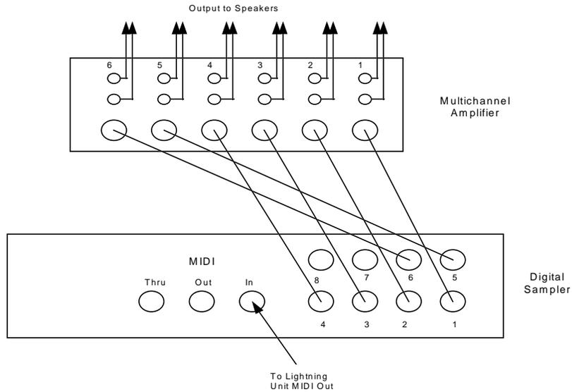
Fig. I-10. Audio Components and Connections
