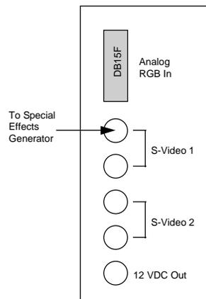
Fig. I-5. Back Panel of Projector
