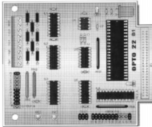
Figure IV-6. Opto22 Brainboard, Model B1
