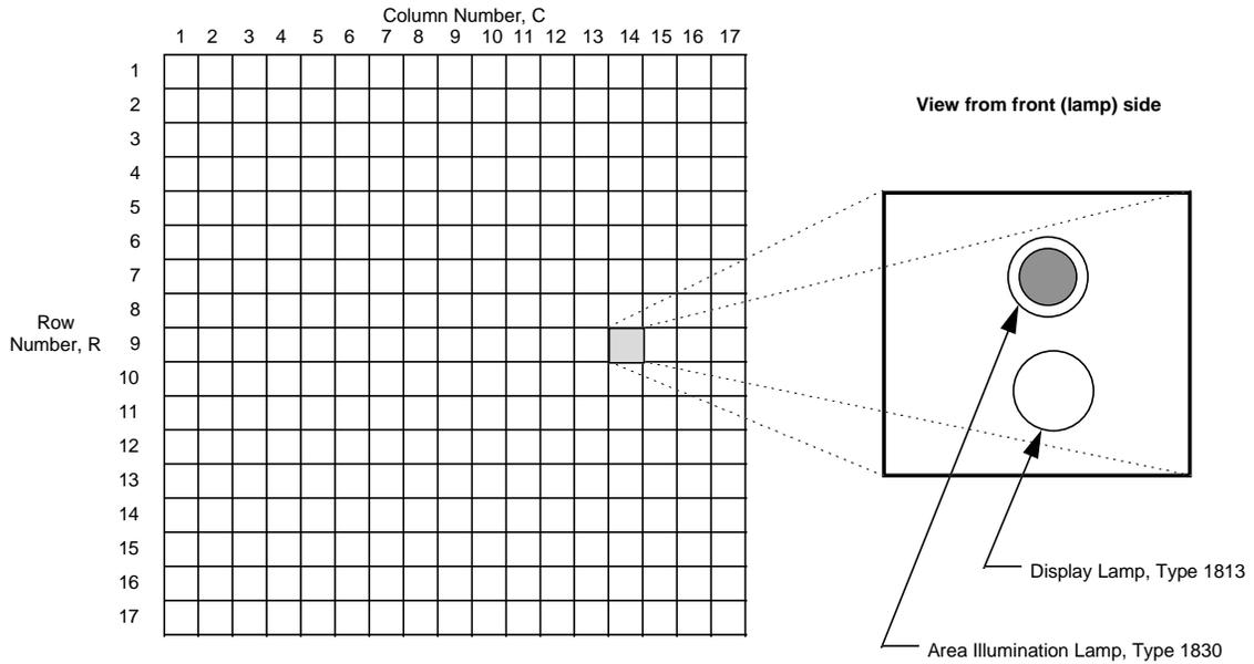
Display lamps are individually addressable. The row driver completes the ground circuit for all lamps in a specified row. The column driver supplies power to all lamps in a specified column.
