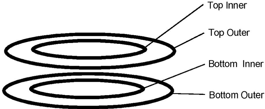
Fig. I-13. Ring Locations on a Single Pan Disc
