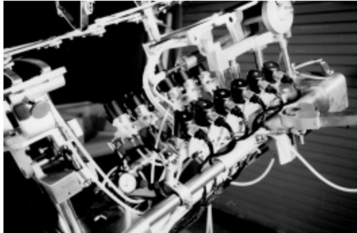
Figure IV-2. Pneumatic Solenoid Valves
