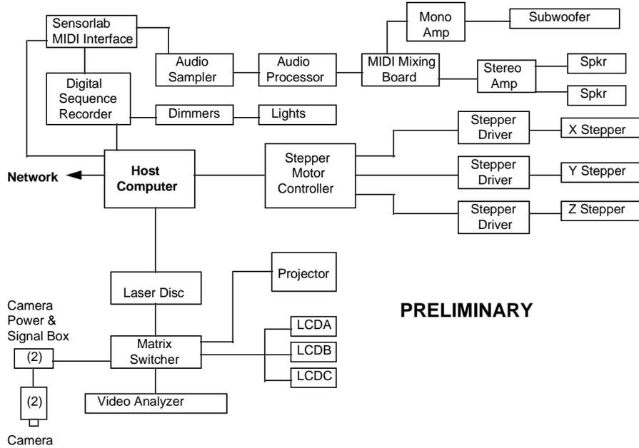
Fig. VI-3. STEALTH System Schematic
