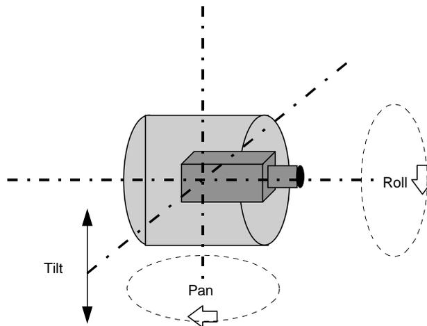
Fig. I-11(a) RPT Head Axes of Motion
