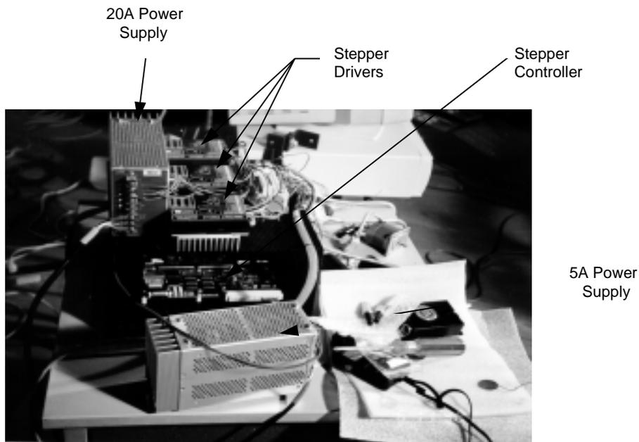
Fig. VI-5. Stepper Motor Drivers and Controller
