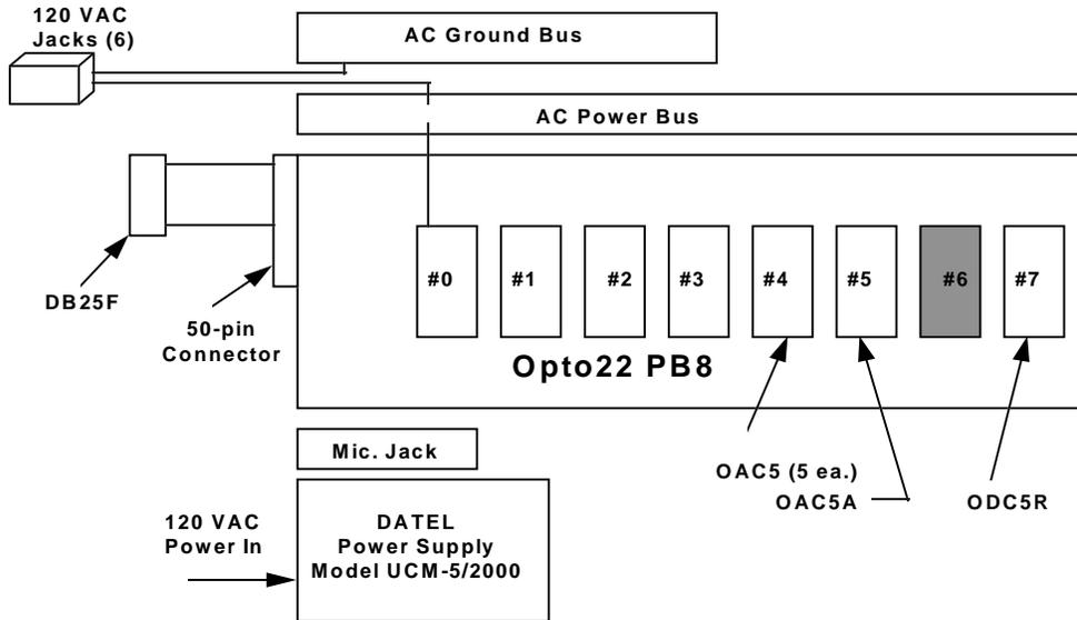
Fig. I-7 Block Schematic, Lighting Controller
