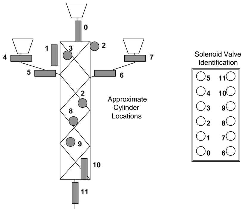
Figure IV-3. Cylinder-Valve Correspondences
