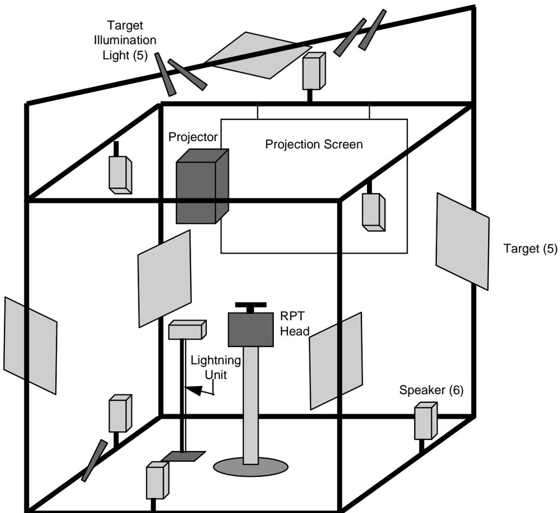
Fig. I-1. Theater of Hybrid Automata Setup
