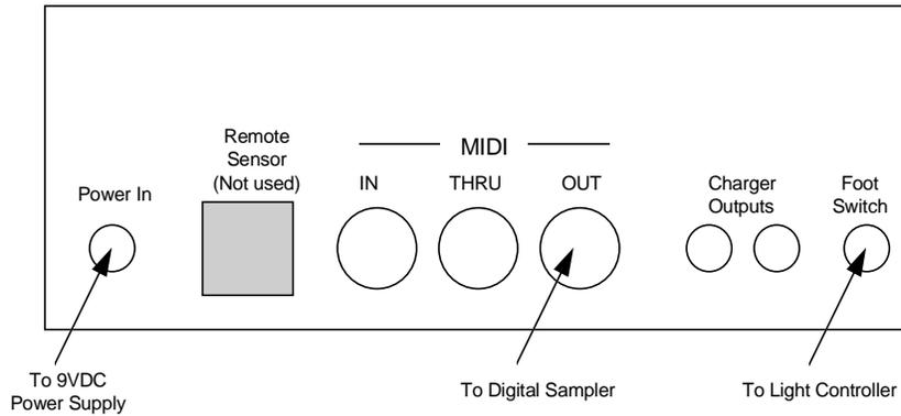
Fig. I-9(b). Back Panel of Lightning Unit
