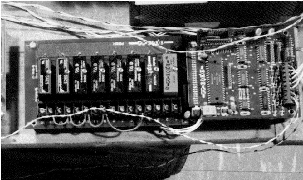
Figure V-4. SCRIBE Relay Board and Brainboard
