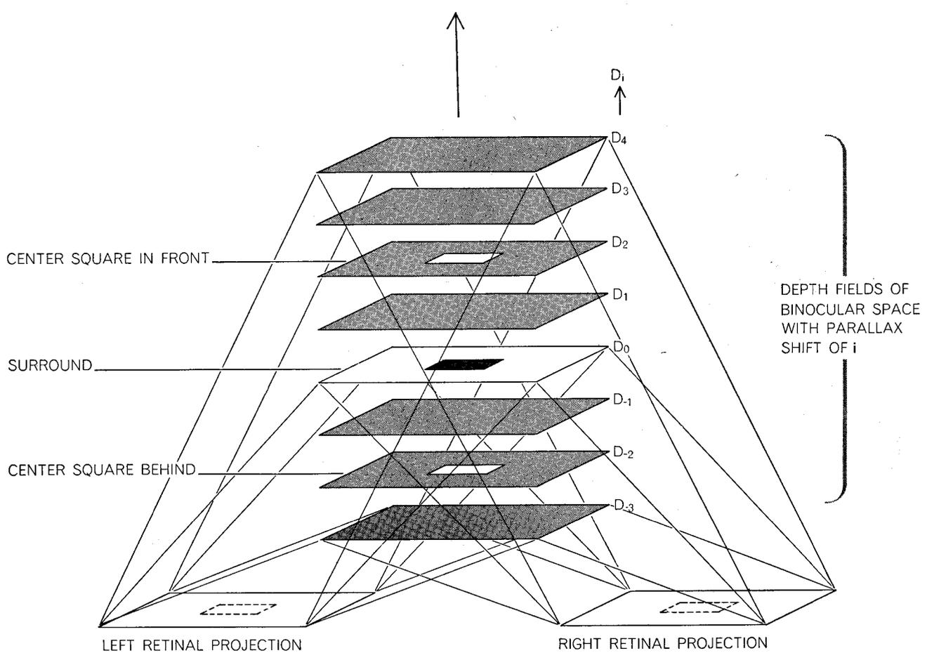
AUTOMAP-1 is a computer program that compiles a three-dimensional contour map from two-dimensional stereoscopic images. The program compares left and right fields point by point and subtracts the brightness of each point from its counterpart. Where the two fields match, the difference is zero, shown above as a white area. Thus the surround ( $D_0$ ) is white except where there
