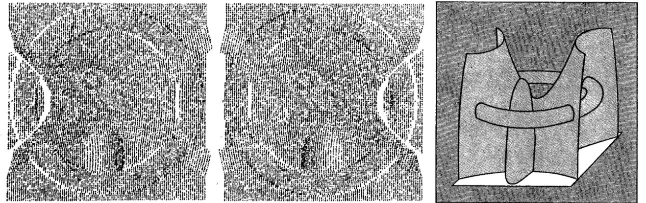
SADDLE-SHAPED FIGURE (far right) was transformed into left and right stereoscopic fields by a computer program devised by the author. The picture elements consist of 64 standard characters randomly selected but paired in the left and right fields.
