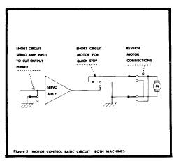
As an additional safety precaution, the inputs to the motor servo amplifiers are shorted to prevent them operating at full power during the switching cycle.
