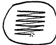
You can usually see the lines clearly on a black-and-white set. The picture consists of the changing pattern of brightness of this beam, which comes in over the airwaves as the television signal.
